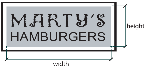
Figure 17.03.080.1. Measurement of sign area.
